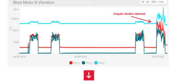
Root cause analysis determined bad shot blades caused imbalance, leading to loosening of the bolts. ATS replaced the shot wheel blades outside of production hours utilizing \$300 worth of in-stock parts.
