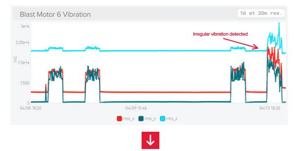
Root cause analysis determined bad shot blades caused imbalance, leading to loosening of the bolts. ATS replaced the shot wheel blades outside of production hours utilizing \$300 worth of in-stock parts.
