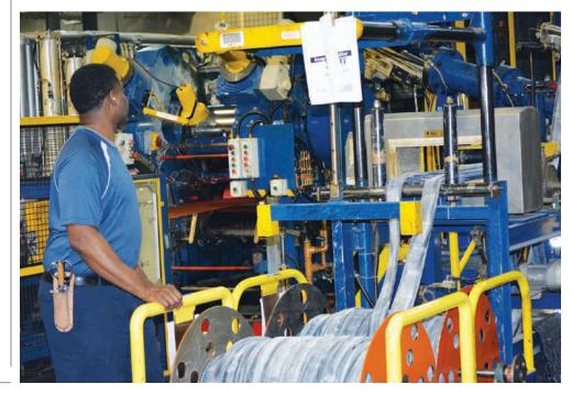
The raw rubber is fed from spools into the first stage of a process that will produce a finished tire, which are stored for distribution in part of Toyo's 3-million sq. ft. plant in White, Ga.
