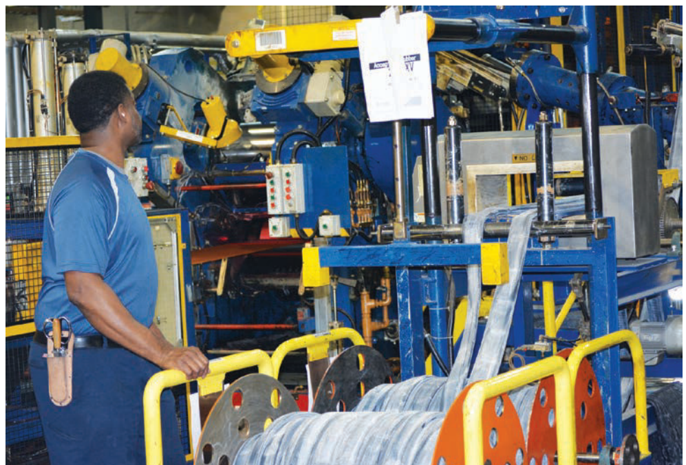
The raw rubber is fed from spools into the first stage of a process that will produce a finished tire, which are stored for distribution in part of Toyo's 3-million sq. ft. plant in White, Ga.
